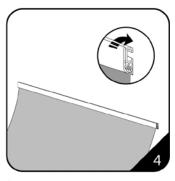
4. Slide the top of the graphic under the lip (it should allow for approx. 3/8" or 1cm insertion) and close the lip to secure the graphic.
