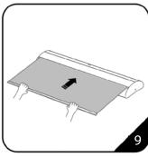
9 .Carefully allow the graphic to recoil into the base unit (it may be useful to have an assistant hold the base steady)
